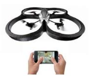
The Drone creates its own Wi-Fi hotspot to which the iPhone or iPod Touch connects. The device gets updates via Wi-Fi as well and has a fairly nice range. Built-in sonar keeps the thing from flying into space.
